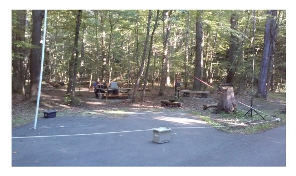
The photo from the first test in the series (Courtesy of Terry Carnahan-KB3JOD) shows the typical setup for the NVIS (white pole) and the 2m antenna at site alpha. Doug is sitting at the table and the radios are provided by Terry C.
